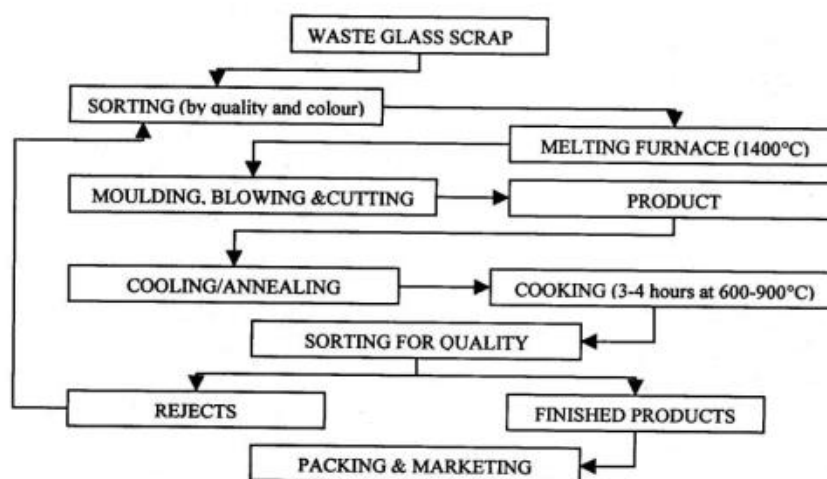
Figure 3.- Glass Processing (Semi-Mechanical)
